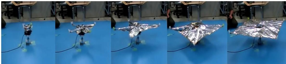
Fig.3 Deployment procedures with cable suspension system.
