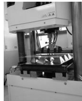
Fig.2 Assembled structures in the bending test.
