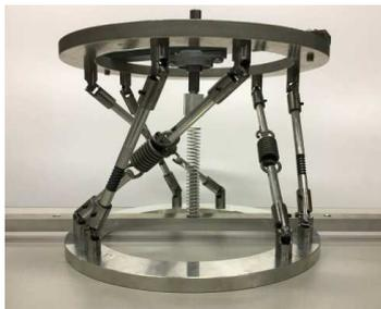
Figure 1 Prototyped vibration isolator. The figure was extracted from [3].
