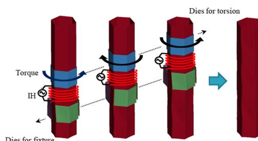
Fig.2 Schematic drawing of the three steps in the torsion forming process: (1) fix the first segment and twist the third segment through a certain angle, thus deforming the second segment; (2) move the dies one segment along the axial direction; (3) repeat step (1), twisting in the opposite direction.
