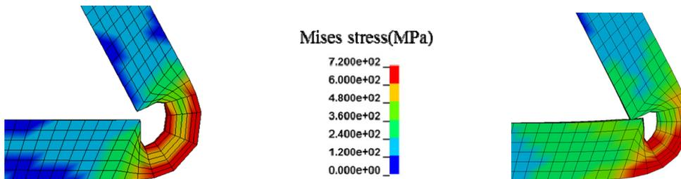
Fig.3 Mises stress distribution of big spring back case.
