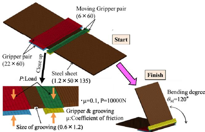
Fig.1 FEM model for gripper bending.
