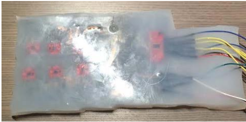
A soft skin that can sense distance and force
